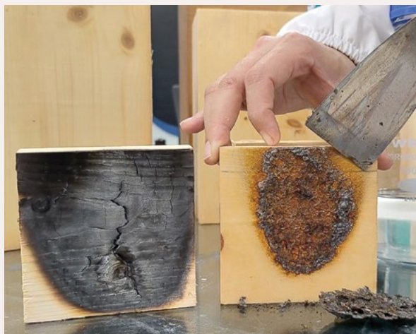
When exposed to fire, wood not coated with the invisible coating (left) gets burnt and damaged, unlike wood protected by the novel coating's char (right). Credit: NTU.
