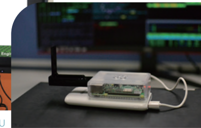
A low-cost, portable, evil twin attack setup invented by the Professors
