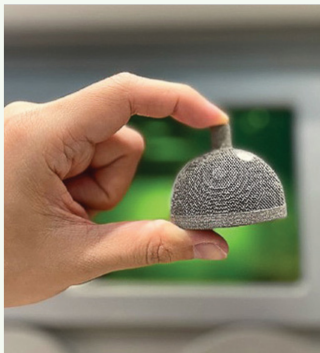
NTU's Singapore Centre for 3D Printing can print orthopaedic implants made from titanium-tantalum that is customised to a patient's unique anatomy, which reduces the amount of surgical time in hospital. Credit: NTU.
