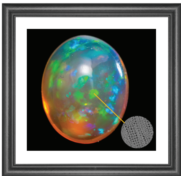
An opal gemstone is a naturally occurring colloidal crystal. The periodicity of its crystalline lattice is comparable to the wavelength of visible light, supplying the jewel's iridescent colors. Micrometer colloidal spheres are like “big atoms”, which can be used to mimic real atomic crystals.
