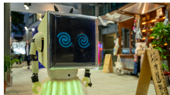
Kevia , 2021, developed by Things That Move, is a full-feature robot that is fully automated, equipped with SLAM (Simultaneous localization and mapping), cameras with face recognition, and a pair of robot arms. Kevia does not serve humans but loves to entertain. It performed as a visitor to entertain on its own during deTour festival.
