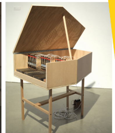
Graphite Piano is a wooden sound instrument, shaped to resemble a piano. Using the pencil as one of the electronic components for generating sounds seems absurd yet completely makes sense because of its physical properties. The pencil core is made of graphite, which enables the pencil to serve as an electrical conductor.
